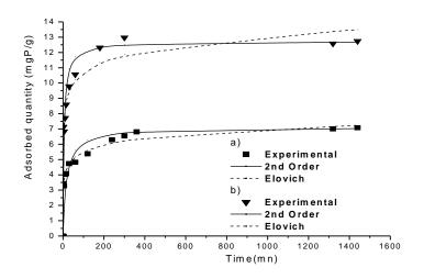
Figure 3: Adsorption kinetics (Hematite dose: 2g/l; phosphate concentration: a) 1mM, b) 2mM; pH: 5)
