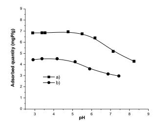
Figure 5: Effect of pH on phosphate adsorption on hematite (Hematite dose: 2g/l; phosphate concentration: a) 2mM, b) 1mM)
