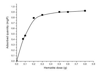
Figure 2: Effect of Hematite dose on phosphates adsorption (pH: 5)
