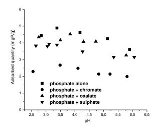
Figure 6: Effect of anions on phosphate adsorption (Hematite dose: 2g/l; phosphate concentration: 1mM; anion concentration: 1Mm)
