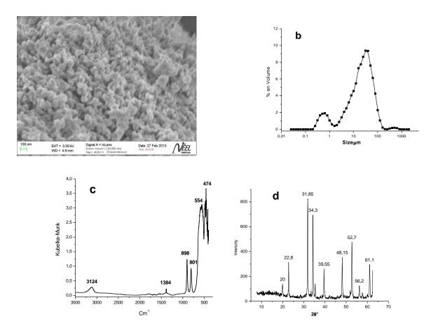
Figure 1: Characterization of the prepared Hematite
